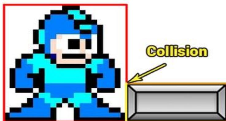
Gambar 3.2 Algoritma Collision Bounding Box(<http://www.kilobolt.com>, 12-06-2016)
