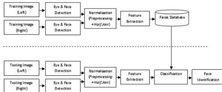
Figure 1. Face Recognition Using Asymmetrical Half-join Method
