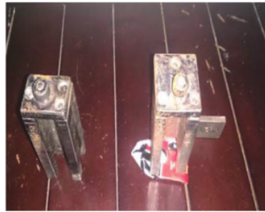
Picture 5 Lock system with adjuster from above
