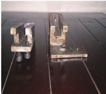
Picture 6 Lock up slot for oscillating shaft locked
