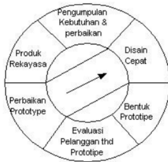
Gambar 4.1. Prototyping Method (Pressman, Roger S.,2002)
